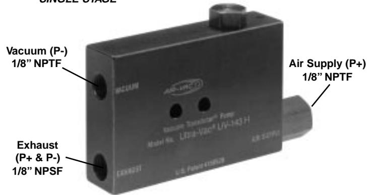
Ultra-Vac's design provides near perfect vacuum of 29.7" Hg. Used to evacuate chambers, degas liquids and in other processes requiring vacuum levels of 1/4" Hg absolute (8 Torr). Ultra-Vac can be used as a first stage in applications requiring high vacuum to reduce operating time of expensive high vacuum pumping systems.
