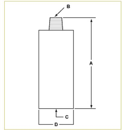
The outer shell is lined with sound absorbing foam for increased noise reduction. It's also constructed entirely of stainless steel to withstand both high temperatures and corrosive environments. They are very easy to install into the exhaust port of vortex tubes, valves, air cylinders, pumps, etc. Expect approximately 23 dBA of noise reduction!
