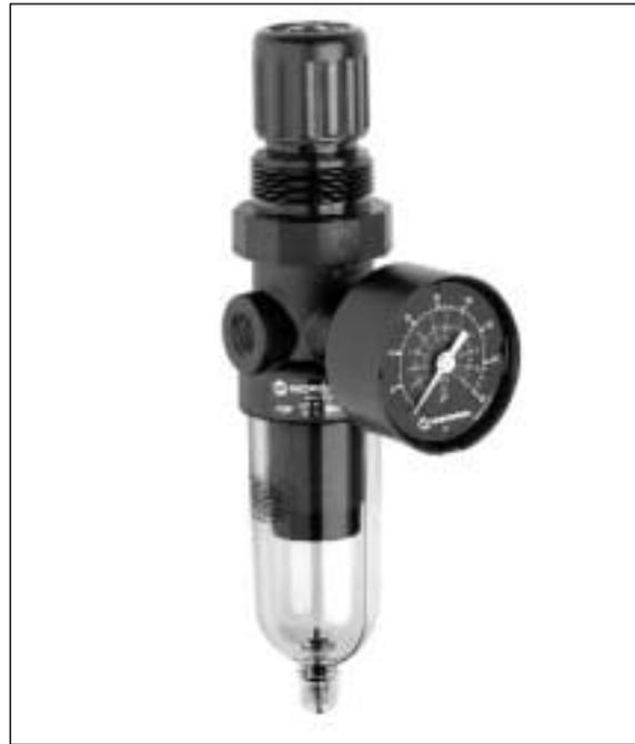
**Ordering Information.** Models listed include PTF threads, transparent bowl, relieving diaphragm, gauge, automatic drain, 5 to 100 psig (0.3 to 7 bar) outlet pressure adjustment range\* .
