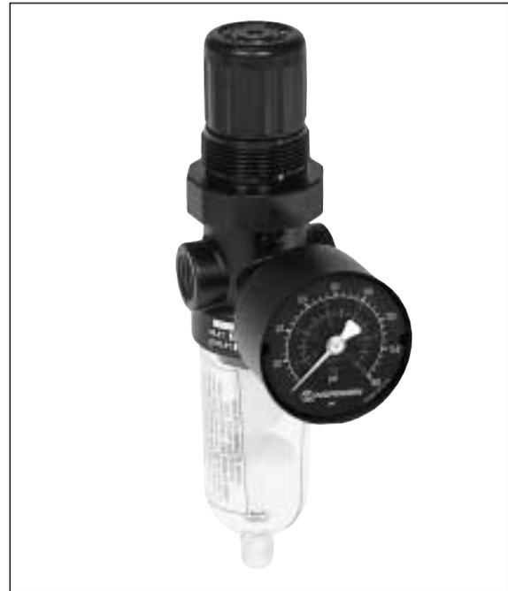
**Ordering Information.** Models listed include PTF threads, transparent bowl, relieving diaphragm, gauge, automatic drain, 5 µm element, 5 to 100 psig (0.3 to 7 bar) outlet pressure adjustment range\*.
