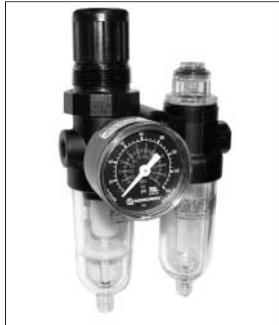
**Ordering Information.** Models listed include PTF threads, transparent bowls, filter/regulator with relieving diaphragm, automatic drain, 5 µm element, 5 to 100 psig (0.3 to 7 bar) outlet pressure adjustment range\*, gauge, and lubricator with auto drain.
