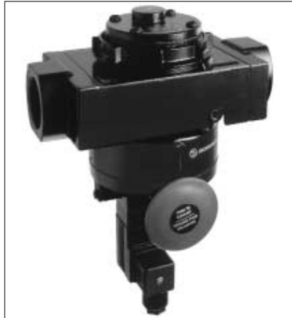
**Ordering Information.** Models listed include a yoke with PTF threads and an operator with manual lockout slide. Solenoid operated models include a 22 mm operator with manual override, a 24 Vdc coil, and a connector without indicator light.
