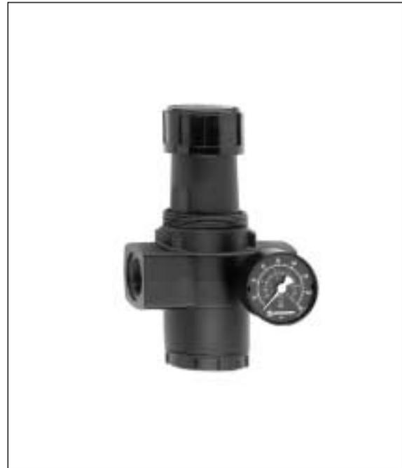
**Ordering Information.** Models listed are knob adjustment, relieving type with gauge, 5 to 125 psig (0.3 to 8.5 bar) outlet pressure adjustment range\*, and PTF threads.
