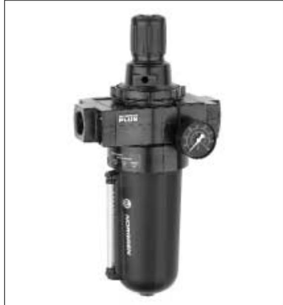
**Ordering Information.** Models listed include a 1 quart w/long element, yoke with PTF threads, knob adjustment, automatic drain, 40 µm element, relieving diaphragm, and a 5 to 120 psig (0.4 to 8 bar) outlet pressure adjustment range\*. A gauge is not included.
