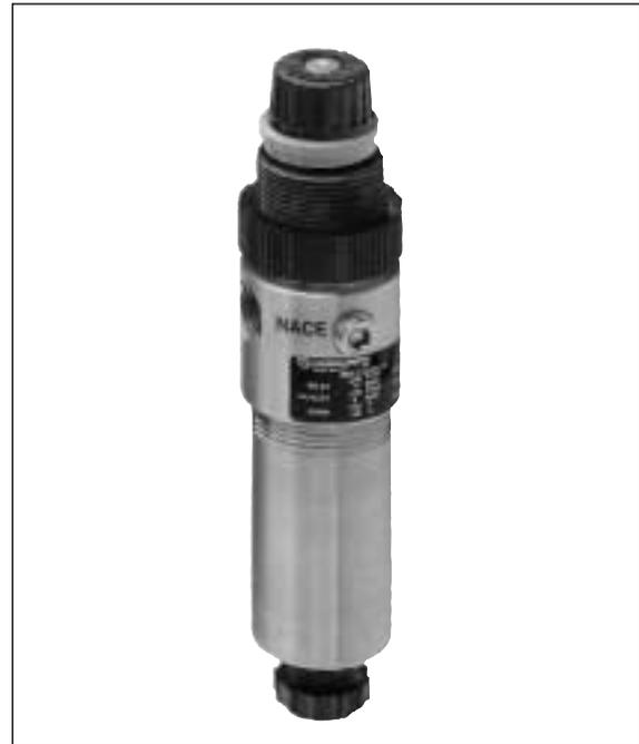
**Ordering Information.** Model listed includes a relieving diaphragm, manual drain, 40 µm element, 5 to 125 psig (0.3 to 8.5 bar) outlet pressure adjustment range\*\* and PTF threads. A gauge is not included.
