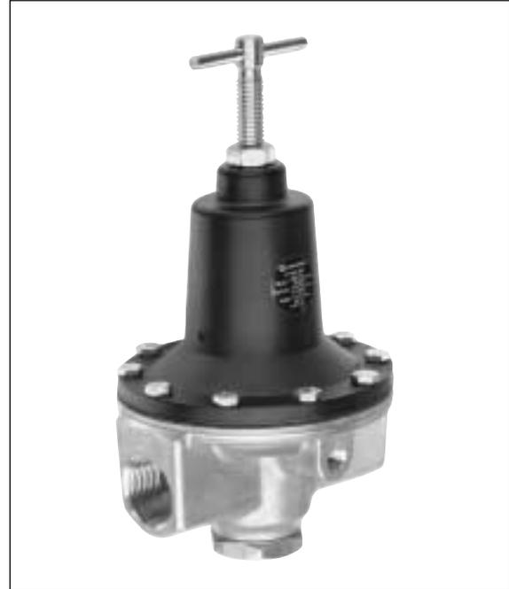
**Ordering Information.** Models listed have PTF threads, T-bar adjustment, non-relieving diaphragm, and 5 to 125 psig (0.3 to 8.5 bar) outlet pressure adjustment range\*. A gauge is not included.
