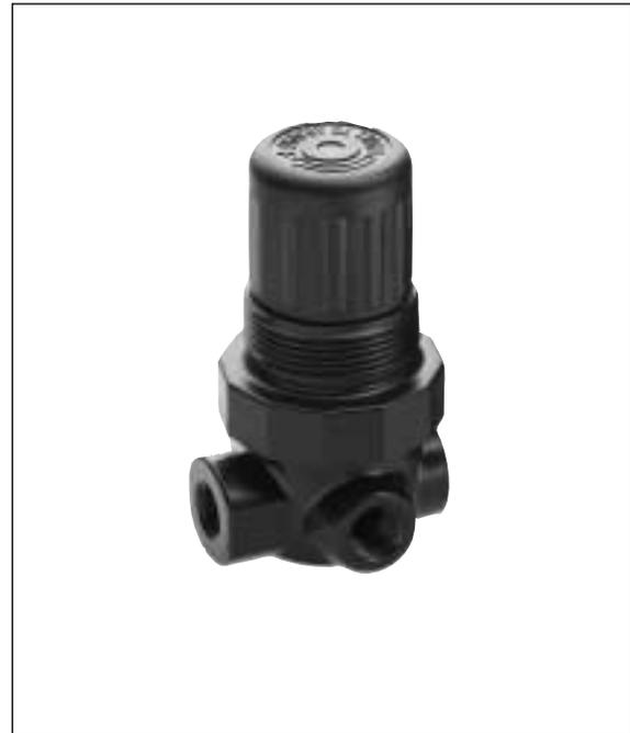
**Ordering Information.** Models listed include PTF threads, knob adjustment, non relieving diaphragm, 5 to 125 psig (0.3 to 8.6 bar) outlet pressure adjustment range†, and without gauge.
