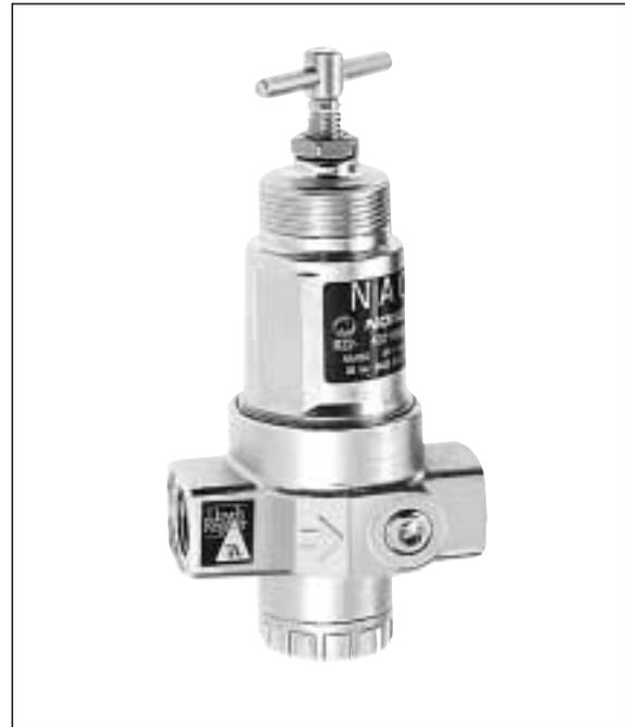
**Ordering Information.** Models listed have T-handle adjustment, relieving diaphragm, 5 to 150 psig (0.4 to 10 bar) outlet pressure adjustment range and PTF threads. A gauge is not included.
