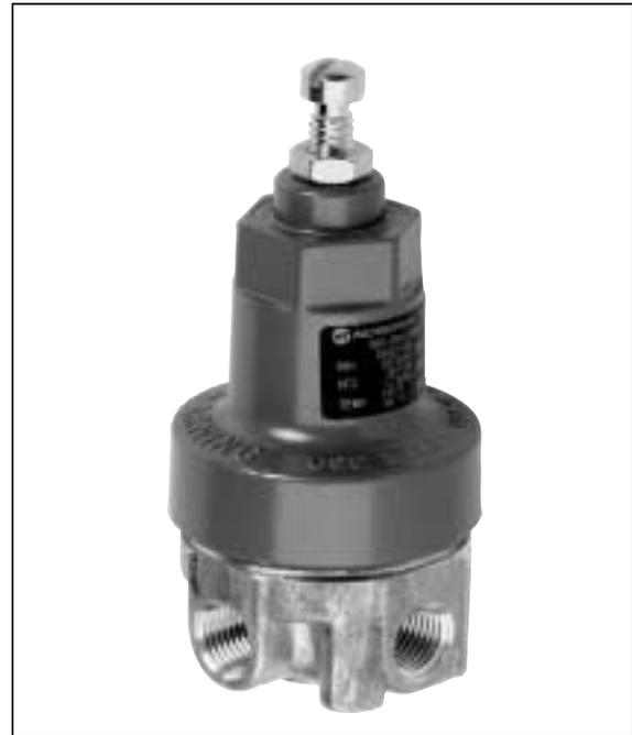
**Ordering Information.** Models listed include PTF threads, relieving diaphragm, 5 to 125 psig (0.3 to 8.5 bar) outlet pressure adjustment range<sup>†</sup>, and without gauge.
