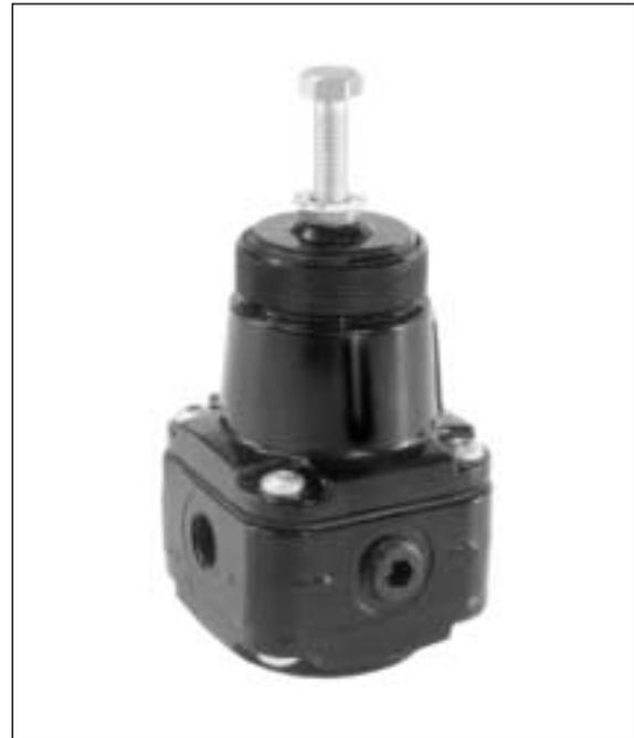
**Ordering Information.** Models listed are relieving type with 0.6 to 30 psig (0.04 to 2 bar) outlet pressure adjustment range \*, and PTF threads. A gauge is not included.
