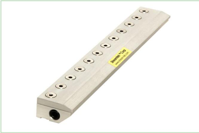
The Advanced Air Knife is an eco-friendly and energy efficient way to clean, cool and dry applications. Without using any electricity or any moving parts, the Advanced Air Knife produces a high velocity, high flow laminar sheet of air by using only a small amount of compressed air as its power source. The Advanced Air Knife provides an amplification ratio of 40:1 and air consumption of 2.9 SCFM per inch at 80 PSIG.
