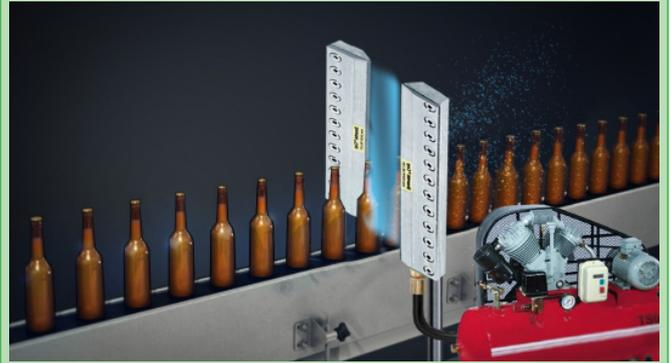
Two (2) **Model AE12SDS-1** Stainless Steel (Type 303) Regular Air Knives are used to blow-off liquid from 1 Litre soda bottles. With the elimination of water, the labels are now able to properly adhere. Before installation of the Air Knives, customer estimated they wasted 3 - 5% of their labels. At thousands of bottles per day, this cost can quickly add up.
