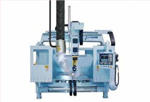
A 1-1/4" Adjustable Air Amplifier (Model - SA-M114A) removes the oily mist from machining operations. This prevents the mist from escaping into the surrounding environment! The Air Amplifier needs no electricity and is compact, making it ideal to mount inside the machine for optimal performance.
