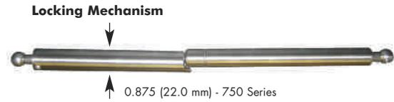
The Locking Mechanism accessory mechanically locks the gas spring in the fully extended position providing assurance of safety. Locking mechanisms are available on the 750 Series gas springs. Adding locking mechanism loses 0.45" stroke. To order add "09" to the part number when ordering. Ex 750-3-XX-09
