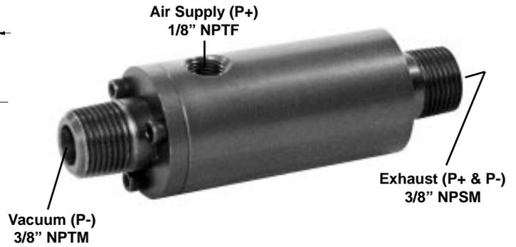
Single Stage design with straight thru vacuum passage is ideal for transporting or conveying solid materials. Simple two piece design has no gaskets or seals to wear.
