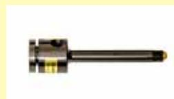
Our Vortex Tube use solid brass generators as their standard generating unit for a longer life expectancy. In higher temperature environments, many competitors will charge an additional fee for this feature. The Streamtek Vortex Tube converts your compressed air supply into a cold airflow at 115°F (46°C) on one end, up to 200°F (93°C) on the other.
